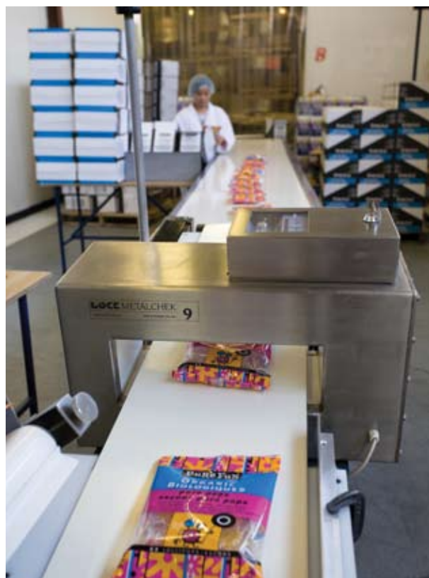
Emerging from the XPdius 800 machine, bags of lollipops pass through the Metal Chek 9 metal detector from Lock Inspection .
